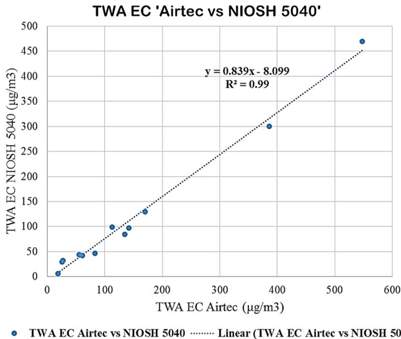
Fig 6. Correlation between shift average EC by Airtec and NIOSH 5040 method
